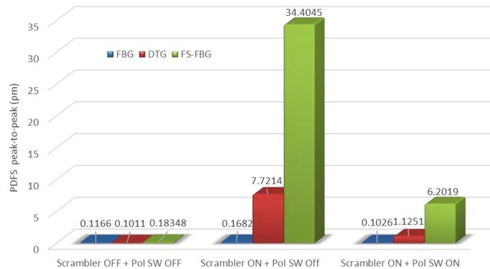
Figure 5. Measured PDFS (peak-to-peak) of the three different FBGs (FBG, DTG, FS-FBG) with a 250Hz LPF applied to all data when the pol. scrambler (emulator) is turned OFF and pol. mitigation OFF (left), pol. scrambler (emulator) is turned ON and pol. mitigation OFF (middle), pol. scrambler (emulator) is turned ON and pol. mitigation ON (right).
