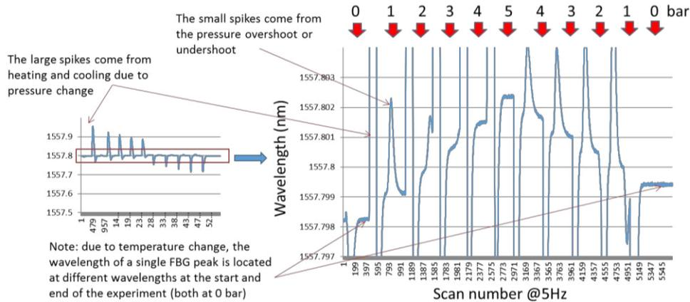
Figure 11. Peak tracking of one of the orthogonal peaks ( $\lambda_1$ ) of the MS-FBG sensor showing the temperature dependency at the start and end of measurement @0bar.
