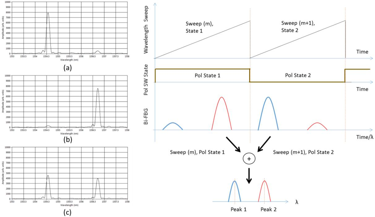
Figure 7. Reflected response from a Bi-FBG for different static polarization states (left), basic operation of the polarization switch in synchronization to the laser sweep to enable spectrum averaging and double peak detection (right).
