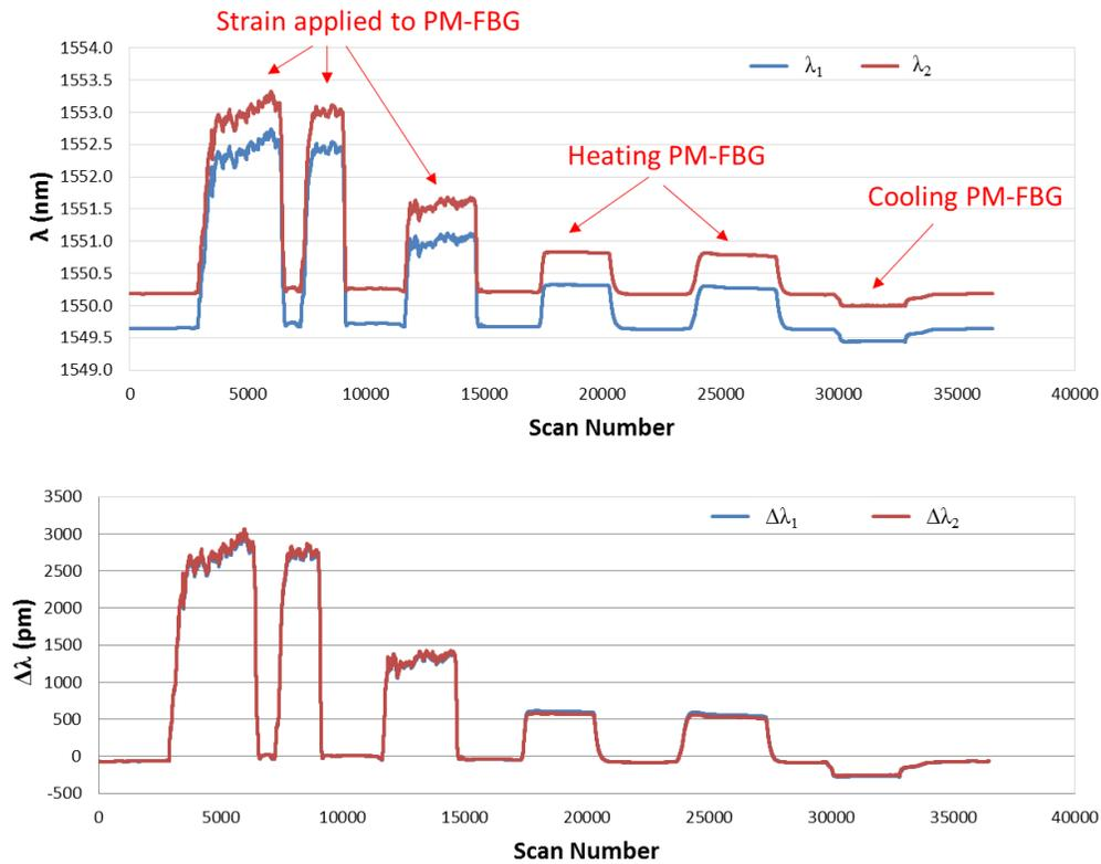
Figure 8. Tracked peaks corresponding to the two orthogonal responses ( $\lambda_1, \lambda_2$ ) of a PM-FBG exposed to strain, heating and cooling with scan rate =250Hz (top), wavelength shift  $\Delta\lambda$  of the orthogonal peaks with respect to their reference  $\lambda$  (bottom).
