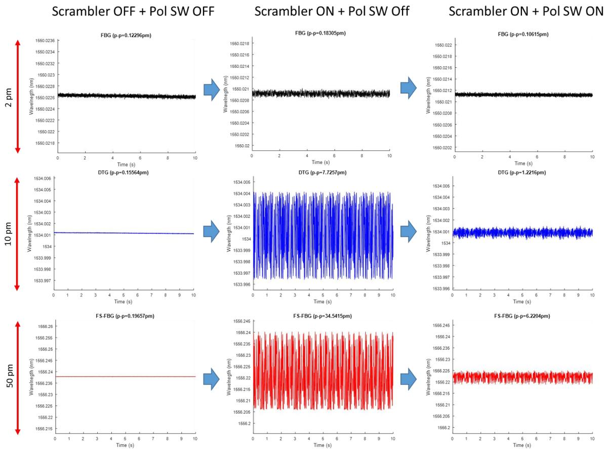
Figure 4. Peak tracking of the three different FBGs (FBG, DTG, FS-FBG) with a 250Hz LPF applied to all data when the pol. scrambler (emulator) is turned OFF and pol. mitigation OFF (left), pol. scrambler (emulator) is turned ON and pol. mitigation OFF (middle), pol. scrambler (emulator) is turned ON and pol. mitigation ON (right).
