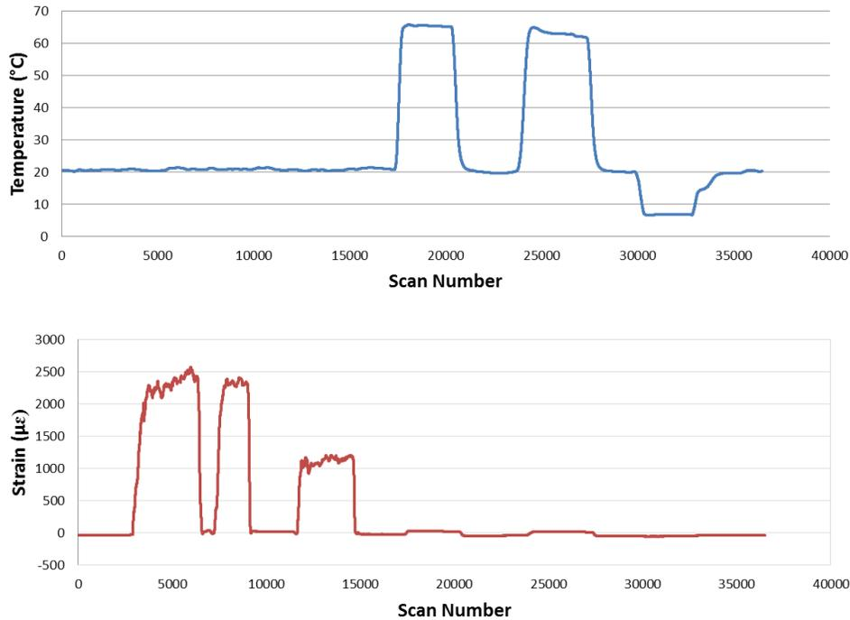
Figure 9. Simultaneous measurement of temperature (Top) and strain (bottom) for the PM-FBG showing the different times where the strain, heating, and cooling was applied to the sensor.
