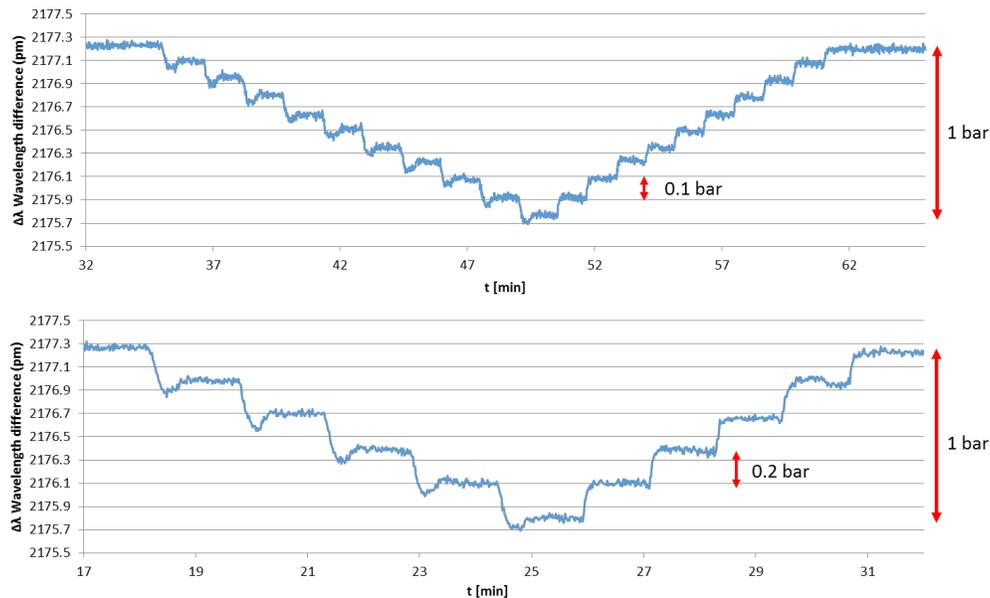
Figure 13. Peak tracking of the two orthogonal peaks ( $\lambda_1, \lambda_2$ ) of the MS-FBG sensor over a 1 bar range using 0.1 bar steps (top), and 0.2 bar steps (bottom).
