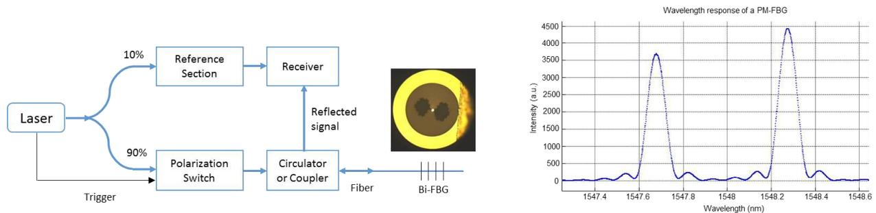
Figure 6. Basic schematic diagram for a single channel FAZT interrogator showing the detection of two birefringent peaks.
