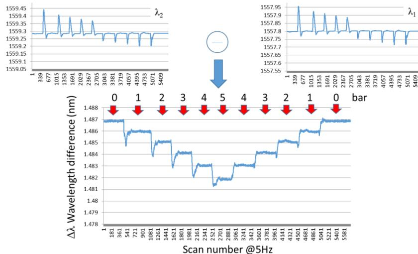
Figure 12. Peak tracking of the two orthogonal peaks ( $\lambda_1$ ,  $\lambda_2$ ) of the MS-FBG sensor (top), wavelength difference between the two orthogonal peaks when the pressured was changed between 0 - 5 - 0 bar in 1 bars steps.
