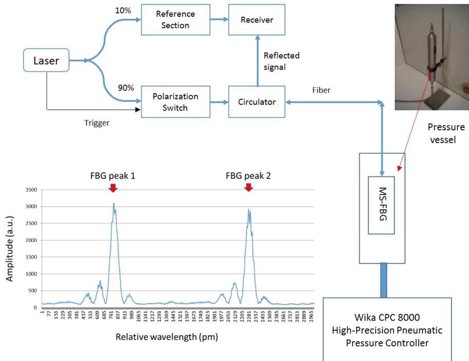
Figure 10. Basic schematic diagram for a single channel FAZT V4 interrogator showing the detection of two birefringent peaks of a MS-FBG pressure sensor installed in a pressure vessel.
