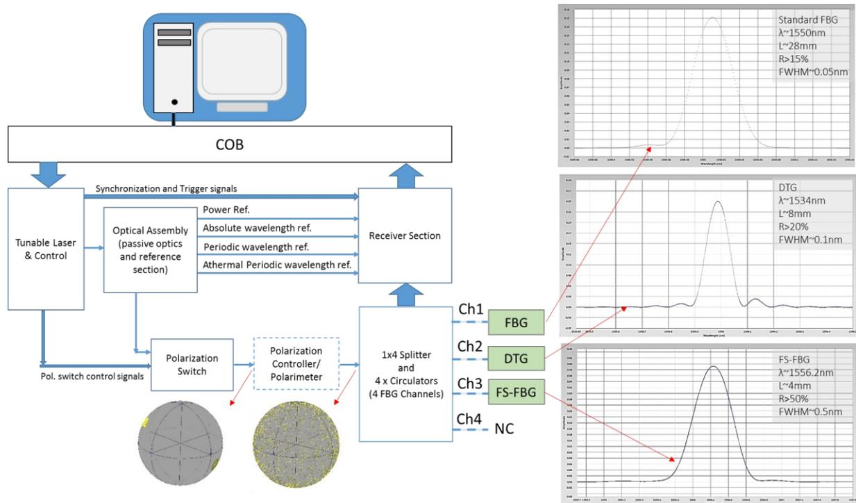
Figure 2. Setup to evaluate PDFS of different type of FBGs using an I4 setup (left). Reflected response and basic specifications of three type of FBGs from different vendors (FBG, DTG, FS-FBG) (right).
